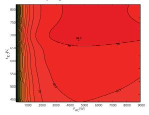
Efficiency characteristic curve for Powador 9.0 TL3
